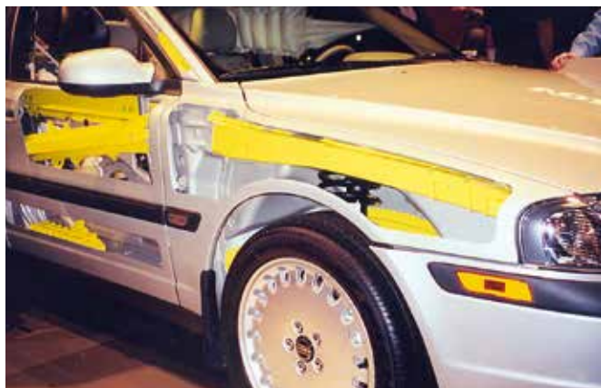
▲ Picture 1. The yellow shaded areas are where the manufacturer has used high strength-low alloy steel.
