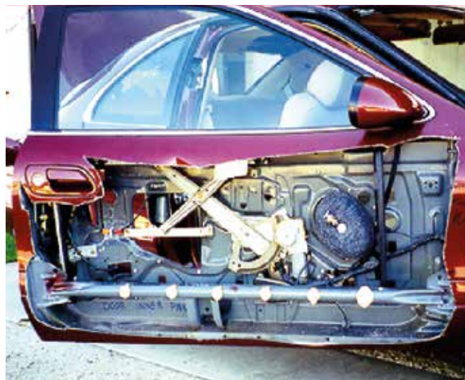
► Picture 2. Ultra high strength steel side impact door beam with a tensile strength of 180,000 psi.
